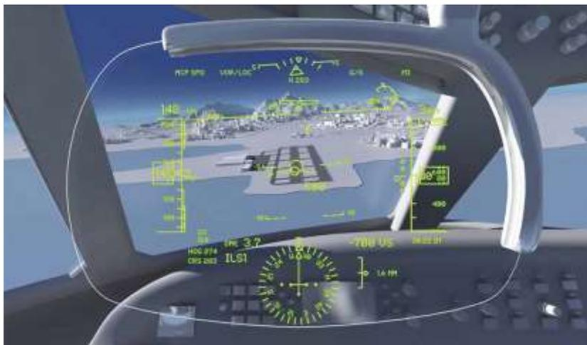
Figure 4 - Head-up Displays (HUDs) in aviation (adapted from <https://www.flyingmag.com/how-it-works-head-up-display/> retrieved on November 20, 2020)
