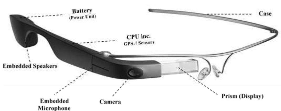
Figure 7 - Basic components of smart glasses (Symbolic illustration of Google Glass 1<sup>st</sup> Generation)
