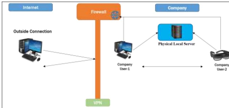
Figure 10 - On-Premise (Local Server) solution for smart glasses
