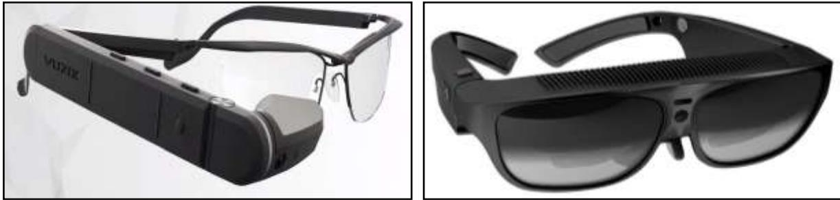
Figure 7 - Vuzix M300 Monocular Smart Glasses (left) & ODG R7 Binocular Smart Glasses (right) (adapted from: <https://www.aniwaa.com/vr-ar/> retrieved on November 21, 2020)
