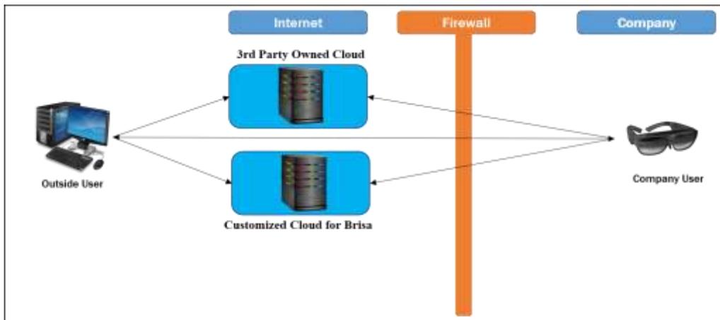
Figure 9 – Cloud solution for smart glasses
